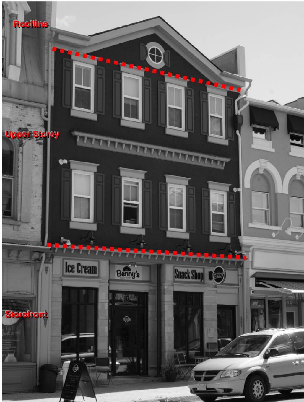
As this example in Downtown Thorold, the traditional definition of façade zone can be accomplished through changes in materials, colours, and architectural elements.
